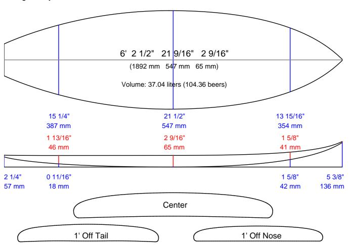
Measurements are center, one foot in and one foot back, over curve.
